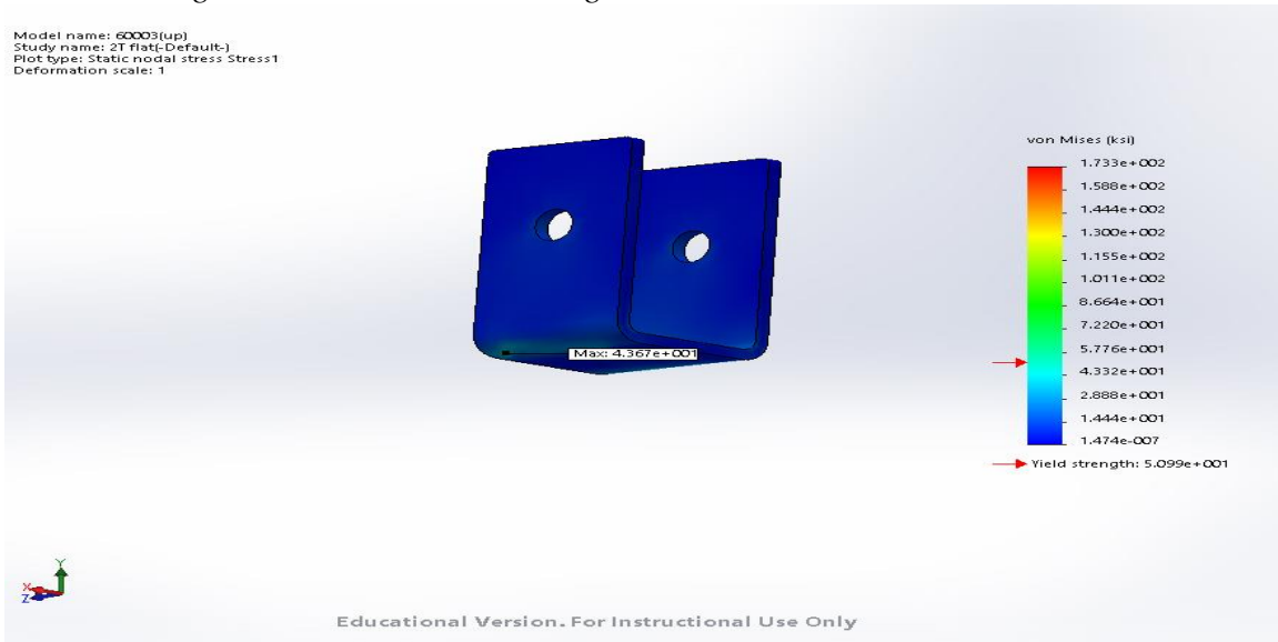
Figure 47: PN#10009 2T Horizontal - Von Mises Stress
