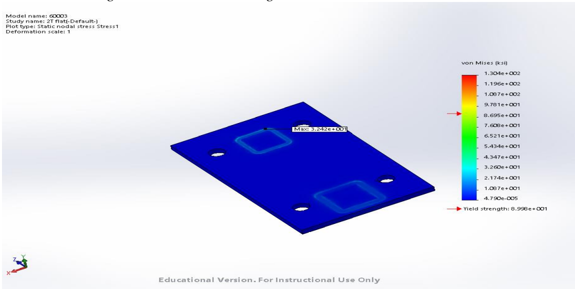
Figure 100: PN#10007 2T Horizontal - Von Misses Stress
