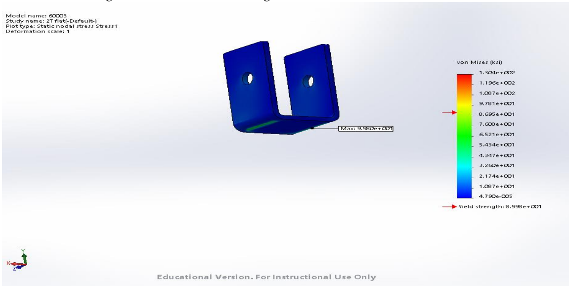
Figure 106: PN#10009 2T Horizontal - Von Misses Stress
