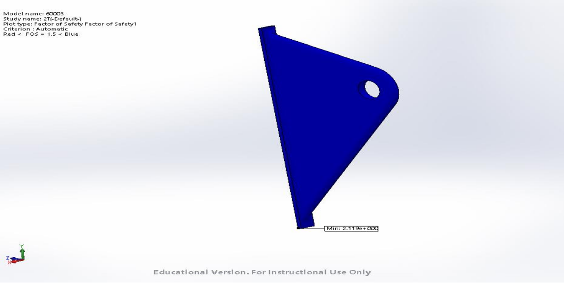
Figure 117: PN#10010 2T Horizontal - F.O.S.
