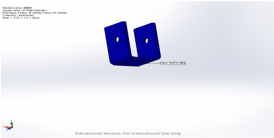
Figure 108: PN#10009 2T Horizontal - F.O.S.
